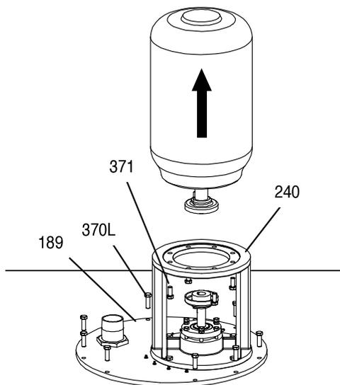
**Figure 23: Motor Bolts Removal**
