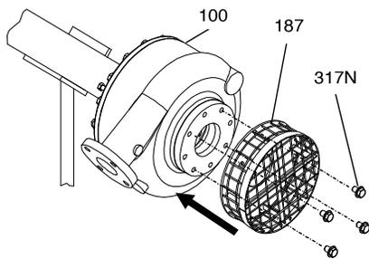
**Figure 46: Strainer reassembly**
