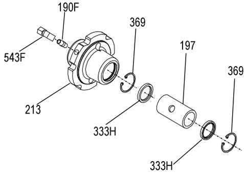
**Figure 38: Steady Bearing Inspection**
