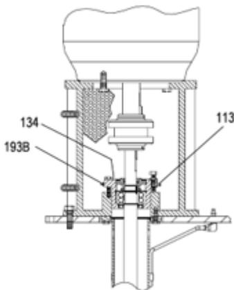
**Figure 21: Thrust bearings**
