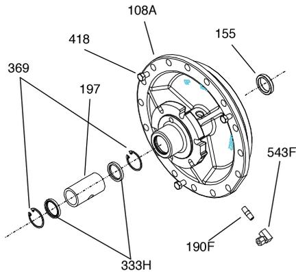
**Figure 41: Steady bearing reassembly**
