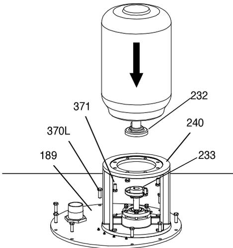
**Figure 47: Motor and coupling reassembly**
