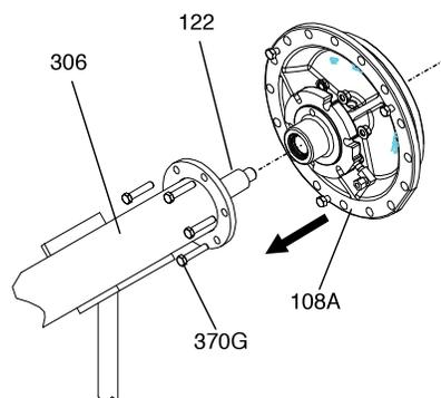
**Figure 42: Adapter reassembly**
