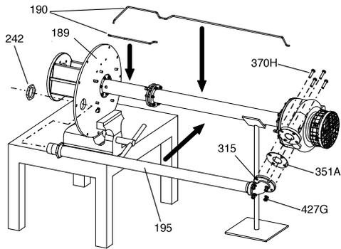
**Figure 45: Discharge pipe reassembly**
