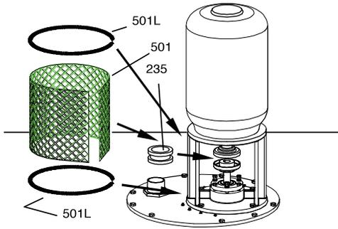
**Figure 48: Coupling guard reassembly**
