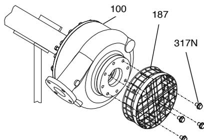
**Figure 25: Strainer removal**
