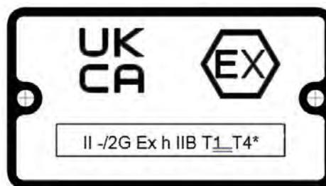
Figure 2: Typical UKCA Ex nameplate
