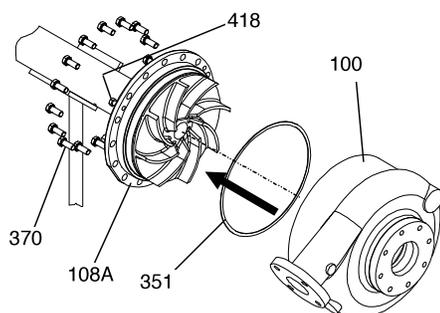
**Figure 44: Impeller adjustment**
