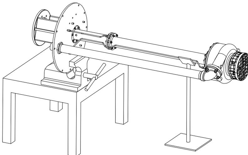
**Figure 24: Lay Pump Horizontally on Proper Supports**
