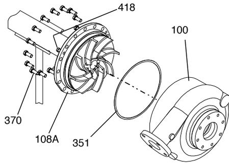
**Figure 26: Casing Removal**
