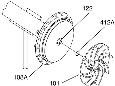
**Figure 29: Impeller Removal**
