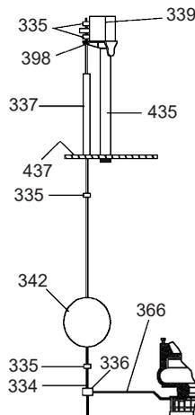
**Figure 15: Radius between float switch column and float**
