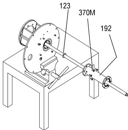
**Figure 32: Head Column Removal**
