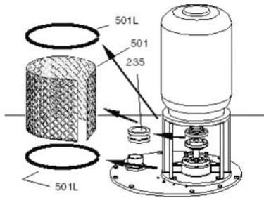
**Figure 22: Coupling Guard Removal**
