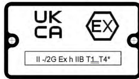
Figure 7: Typical UKCA Ex nameplate
