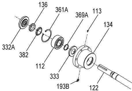
**Figure 34: Labyrinth Seal Removal**
