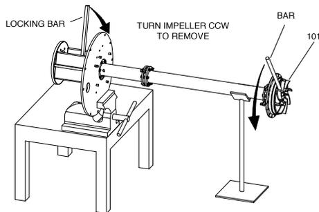
**Figure 28: Impeller Removal**
