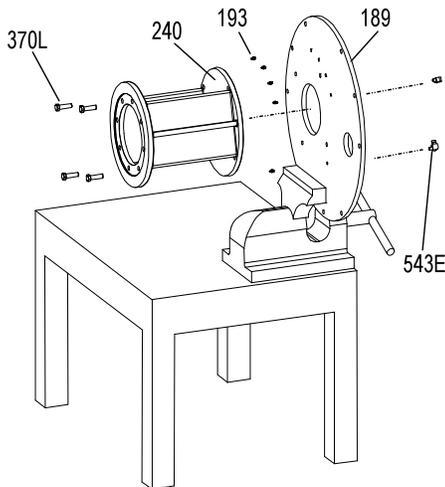
**Figure 35: Motor Adapter Removal**
