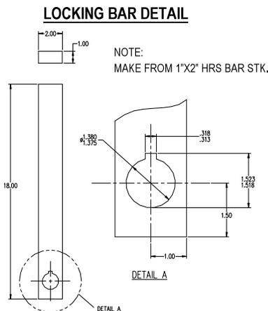
**Figure 27: Locking Bar Detail**
