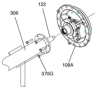
**Figure 30: Adapter Removal**
