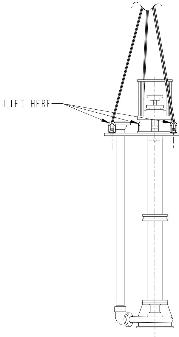
**Figure 4: Example of lifting pump properly with sling**
