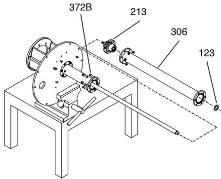
**Figure 31: Column Removal**
