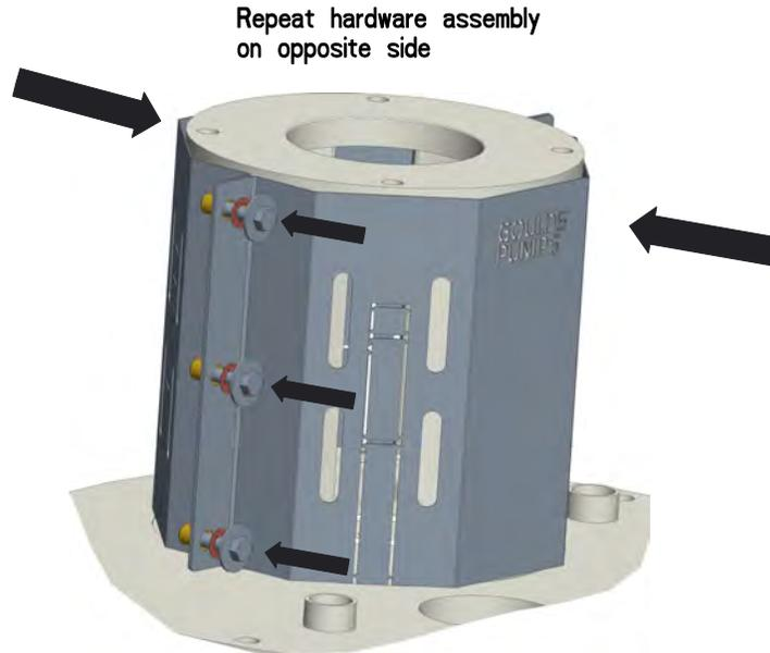
1. Ensure that the mounting bolt for each shaft guard half is inserted with the bolt retainer in place for captive hardware.
