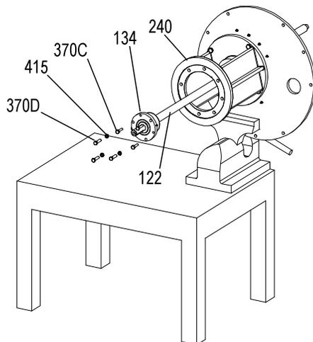
**Figure 33: Bearing Shell and Shaft Removal**
