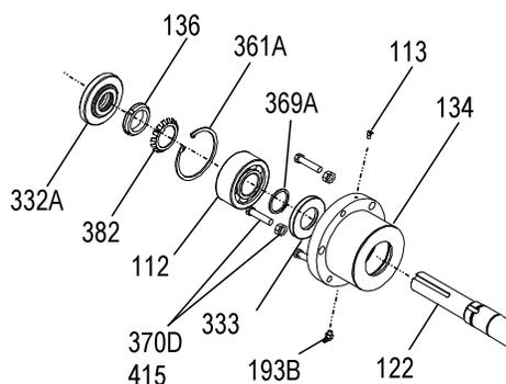
**Figure 39: Retainer ring reassembly**
